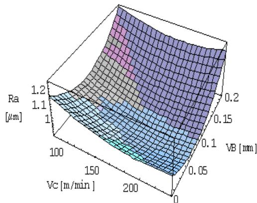
**Fig. 7.** Roughness surface variation with cutting speed and flank wear
