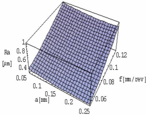
**Fig. 6.** Roughness surface variation with depth of cut and feed rate
