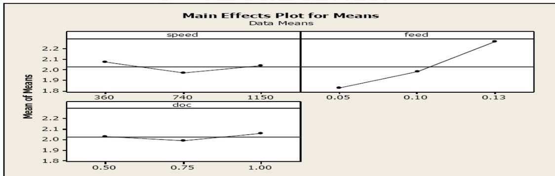
Effect of Turning Parameters on Surface Roughness
