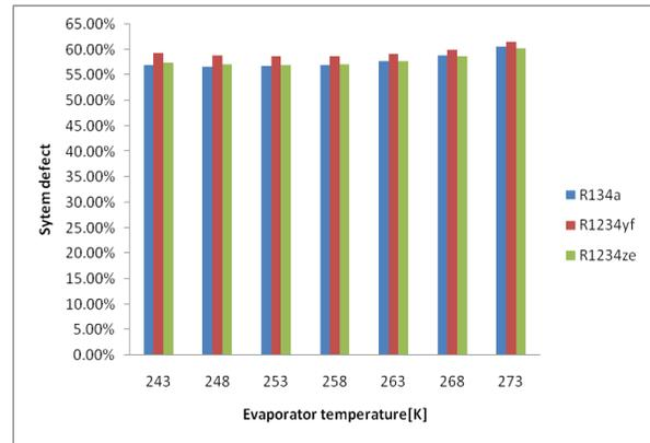
Fig. 4. Variation of system defect with evaporator temperatures
