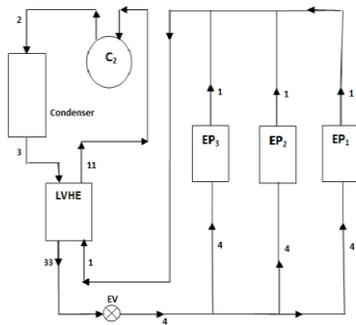
**Fig: 1 (a).** Schematic diagram of actual multievacaporator with single compressor and single expansion valve and LVHE
