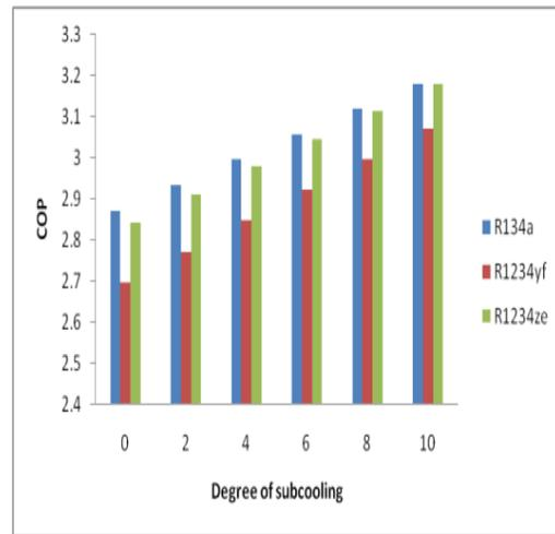
Fig. 5. Variation of COP with degree of subcooling at condenser outlet
