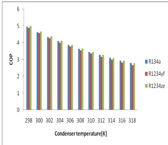
Fig: 7. Variation of COP with condenser temperature
