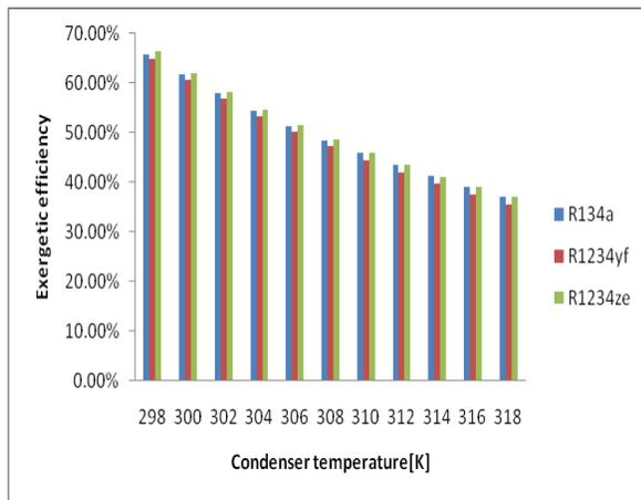
Fig: 8. Variation of exergetic efficiency with condenser temperature Conclusion
