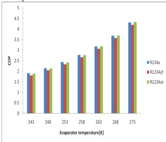
Fig. 2. Variation of COP with evaporators' temperatures
