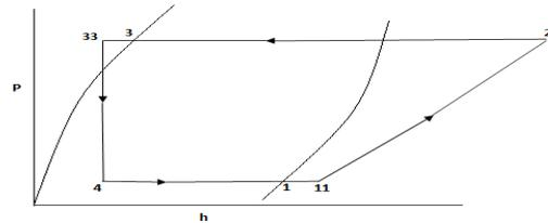
**Fig:1 (b).** Pressure enthalpy diagram of actual multi evaporator with single compressor, and single expansion valve and LVHE
