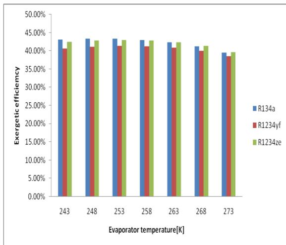
Fig. 3. Variation of exergetic efficiency with evaporators' temperatures
