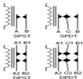
**Fig: 3.** Circuit symbols of relays
