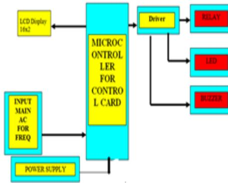
**Fig. 1.** Block Diagram of Under/Over Frequency Relay
