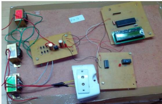
Fig. 3. Picture of Under/Over Frequency Relay
