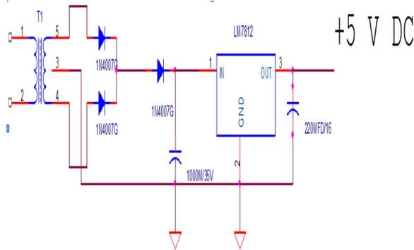
The power supply circuit consists of a bridge rectifier with shunt capacitance filter. A 5 volts regulated source is used for the entire circuit. Three terminal voltage regulators IC 7805 is used to provide 5 volts supply.
