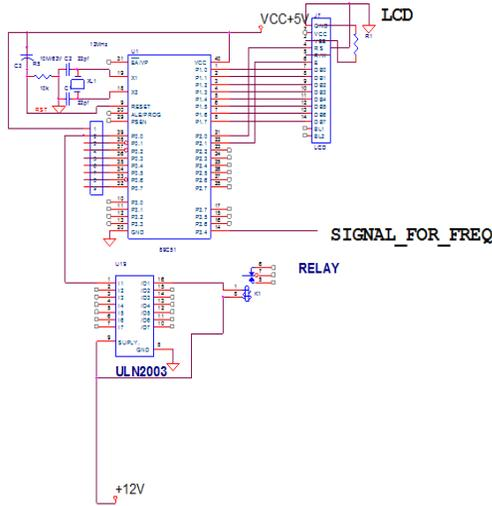
Fig. 2. Circuit Diagram of Under/Over Frequency Relay
