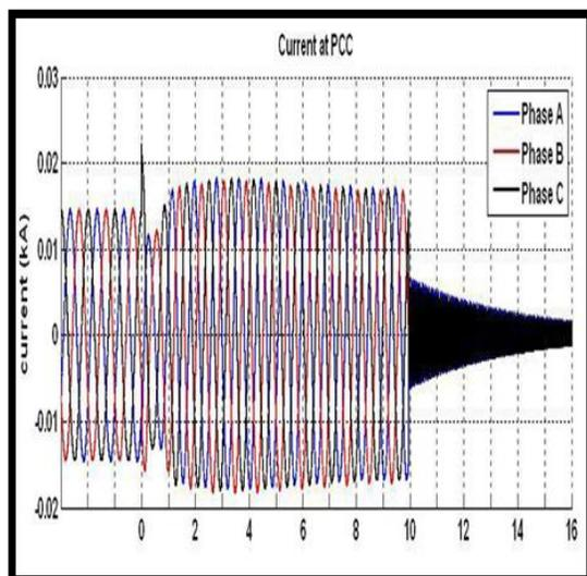
**Fig. 2.** Inverter currents during a three-phase fault close to PCC – Generic Model (time in cycles)
