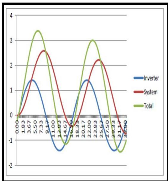
**Fig: 4.** Example of total fault current comparison (assuming one per unit rated inverter current on system base)
