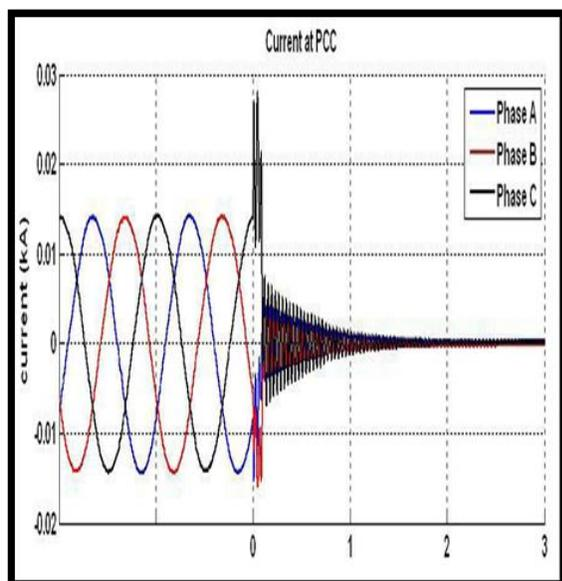
**Fig. 1.** Inverter currents during a three-phase fault close to PCC – Model 1 (time in cycles)
