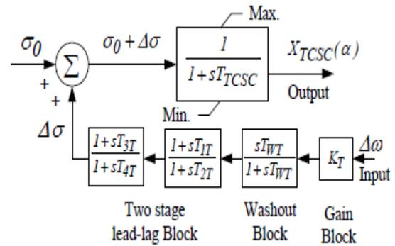
Fig: 2. Structure of TCSC-based controller
