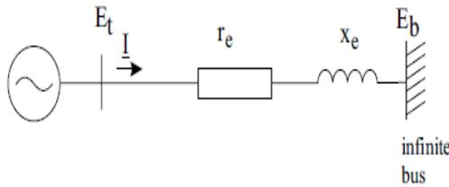
Figure 1: One machine to infinite bus system
