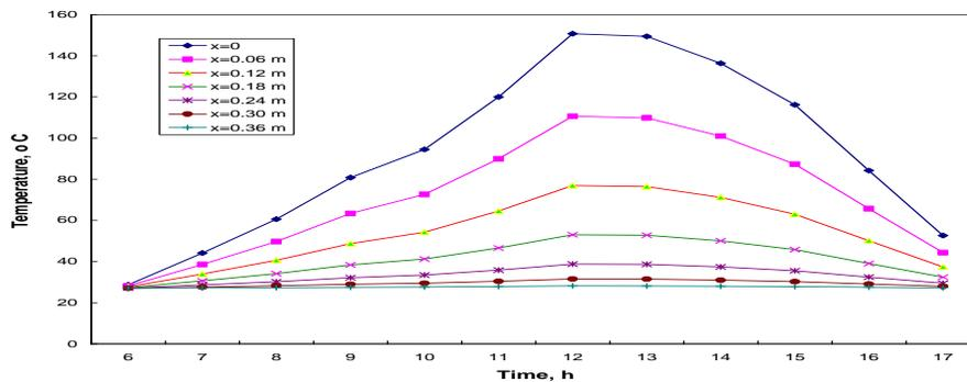
**Fig: 14.** Variation of Temperature across Wall Thickness for Brick Wall
