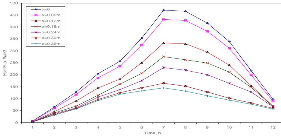
Fig: 18. Variation of Heat Flux with Wall Thickness across Brick Wall
