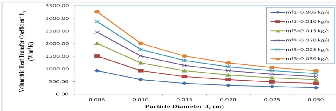
**Fig. 7.** Variation of Volumetric Heat Transfer Coefficient with Particle Diameter for different Mass flow Rates of air
