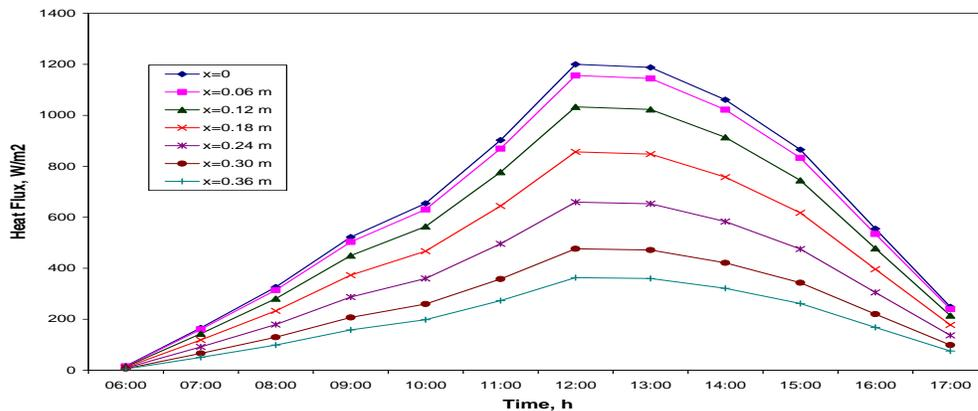
Fig: 20. Variation of Heat Flux with Wall Thickness across Marble wall
