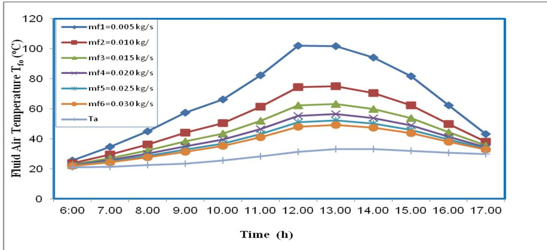
**Fig. 6.** Variation of Fluid (Air) Temperature for different Mass Flow Rates of air and Ambient Temperature with Time of the day
