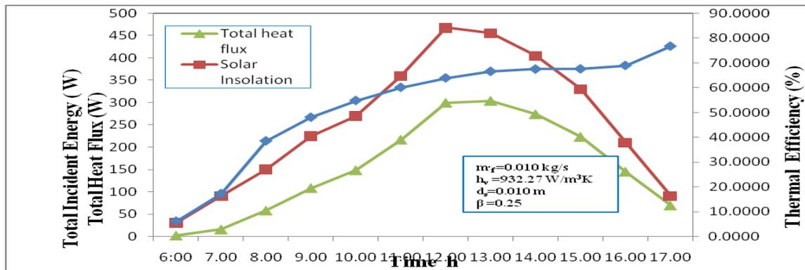
Fig: 11. Variations of Total Incident Energy, Total Heat Flux and Thermal Efficiency for Porous Marble wall with Time of the day at  $x=0.24$  m
