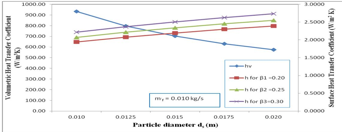
Fig. 9. Variations of Volumetric Heat Transfer Coefficient and Surface Heat Transfer Coefficient with Particle Diameter for different Porosities and a given Mass Flow Rate of air for Porous Marble walls
