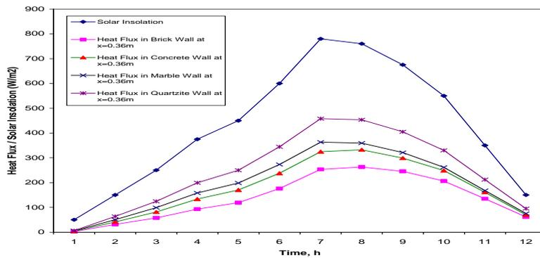
Fig: 23. Variation of Heat Fluxes in Brick, Concrete, Marble and Quartzite Walls at x=0.36 m and Solar Insolation with Time of the day
