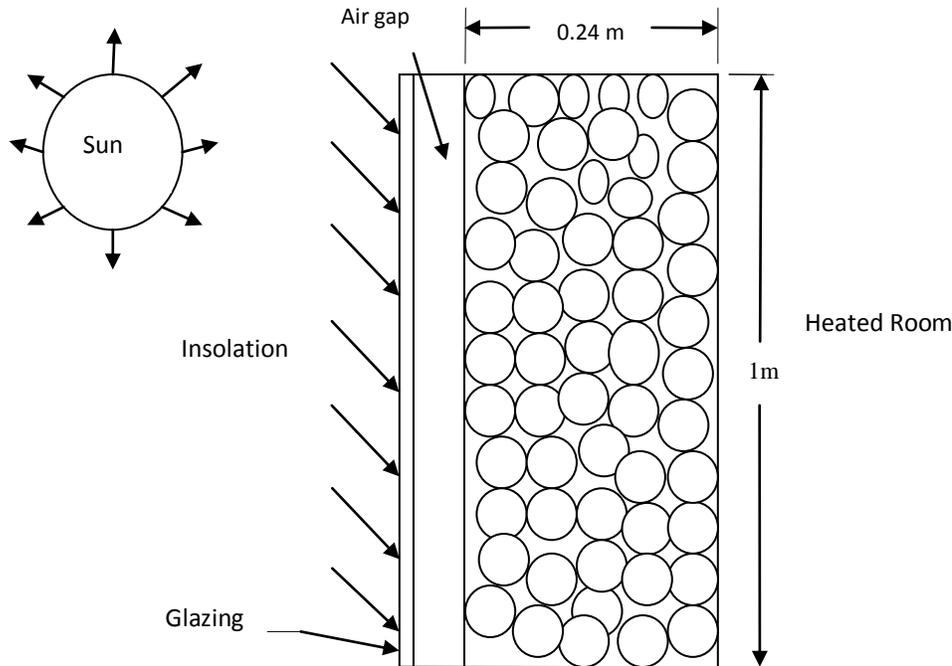
**Fig: 2.** Schematic diagram of a porous wall
