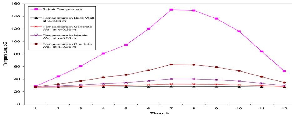
Fig: 22. Variation of Sol-air Temperature and Temperatures in Brick, Concrete, Marble and Quartzite Walls at x=0.36 m with Time of the day
