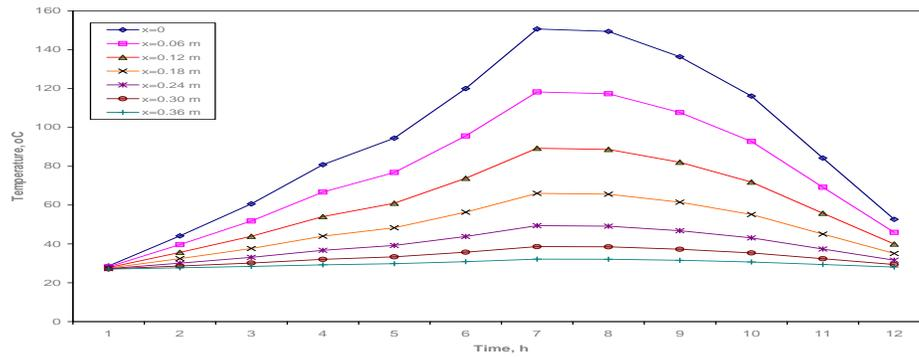
Fig: 15. Variation of Temperature across Wall Thickness for Concrete Wall
