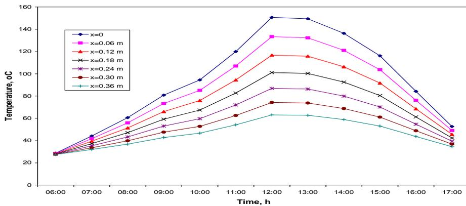
Fig: 17. Variation of Temperature across Wall Thickness for Quartzite Wall
