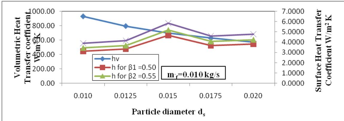
Fig. 10. Variations of Volumetric Heat Transfer Coefficient and Surface Heat Transfer Coefficient with Particle Diameter for different Porosities and a given Mass Flow Rate of air for Porous Quartzite walls
