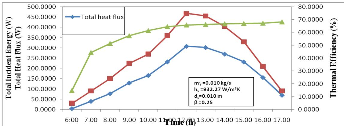
Fig: 12. Variations of Total Incident Energy, Total Heat Flux and Thermal Efficiency for Porous Quartzite wall with Time of the day at  $x=0.24$  m
