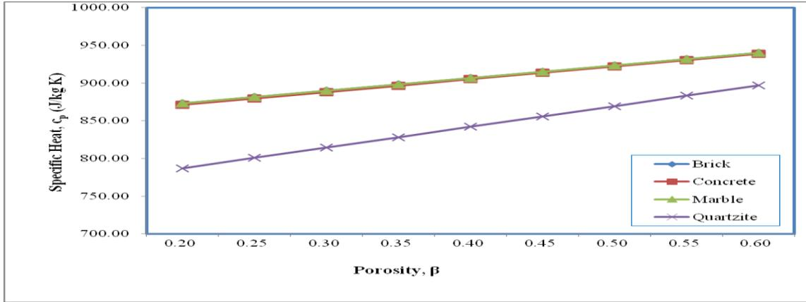
Fig: 3. Variation of Specific Heat with Porosity for different materials
