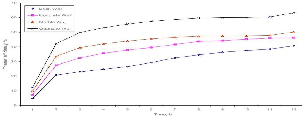
Fig: 24. Variation of Thermal efficiency with Time of the day for different wall materials
