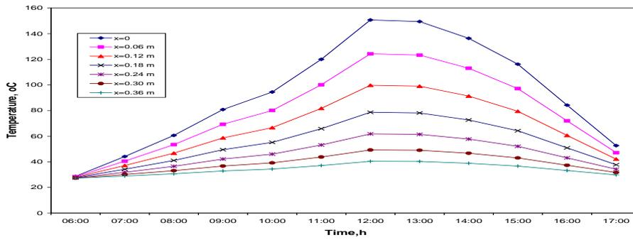
Fig: 16. Variation of Temperature across Wall Thickness for Marble Wall
