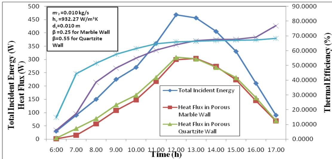
Fig: 13. Comparison between the variations of Total Incident Energy, Heat Fluxes and Thermal Efficiencies of Marble and Quartzite walls with Time of the day at  $x=0.24 \text{ m}$
