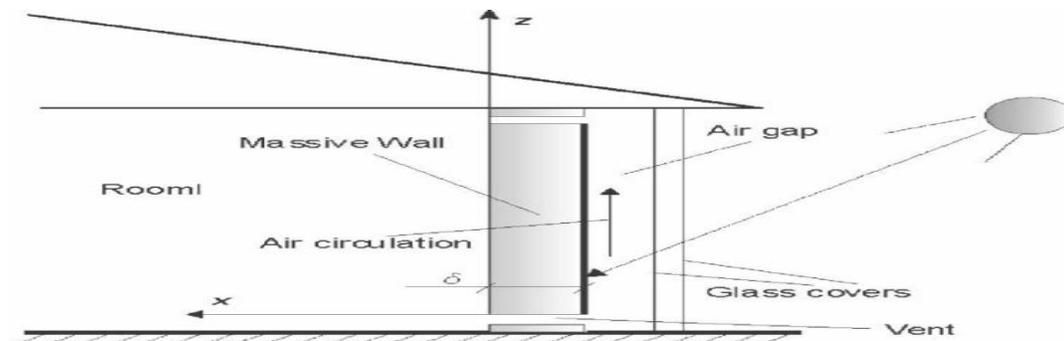
**Fig. 1.** Schematic diagram of 'Trombe Wall' System [1]
