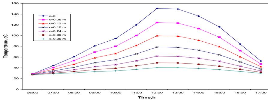
Fig: 16. Variation of Temperature across Wall Thickness for Marble Wall
