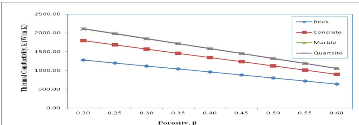
Fig: 5. Variation of Thermal Conductivity with Porosity for different materials
