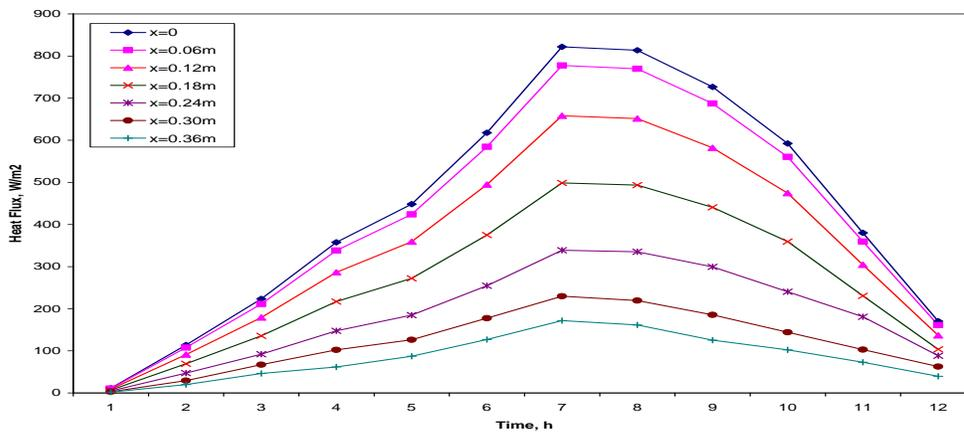
Fig. 19 Variation of Heat Flux with Wall Thickness across Concrete Wall
