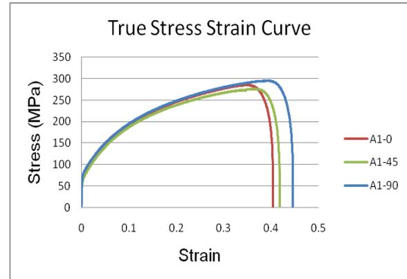
**Fig: 2.** True Stress Strain Curve for IF Steel
