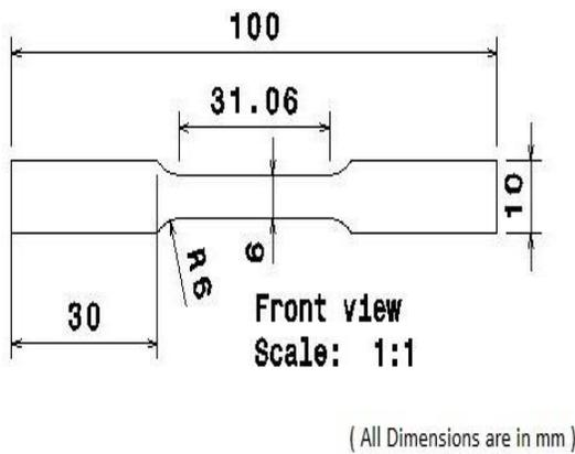
**Fig: 1.** Sample Size according to ASTM E8M-04 tested in UTM
