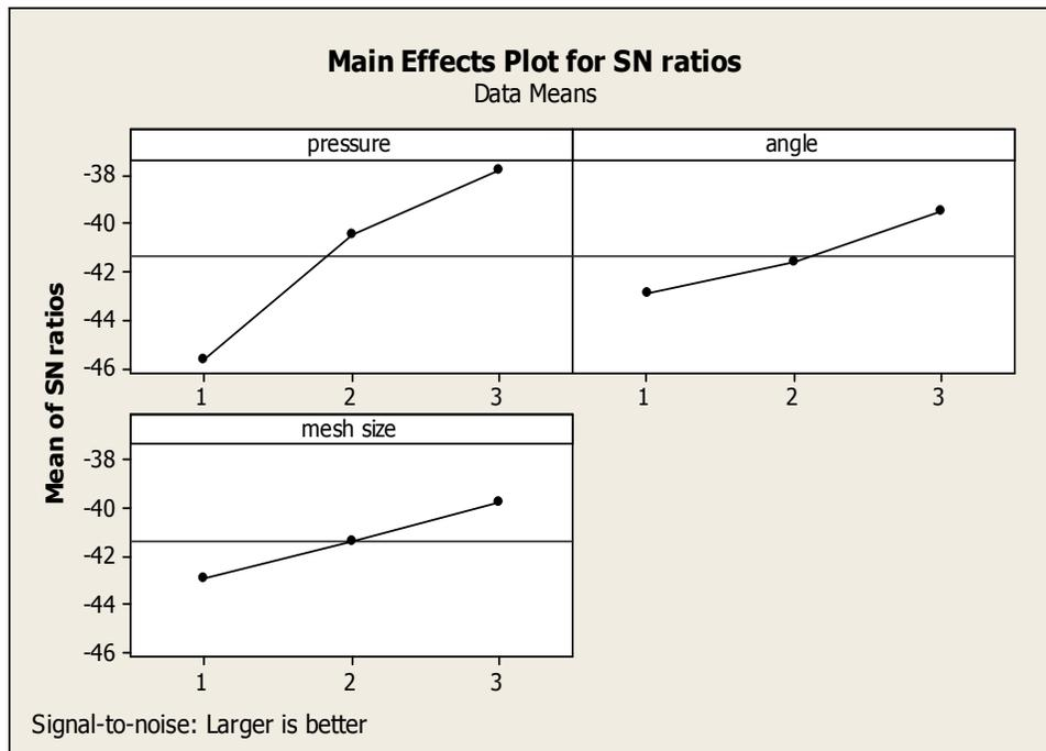
**Fig. 1.** Graph showing S-N Ratio, Larger is better
