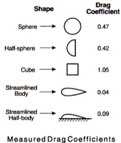
Fig: 3 Measured drag coefficient
