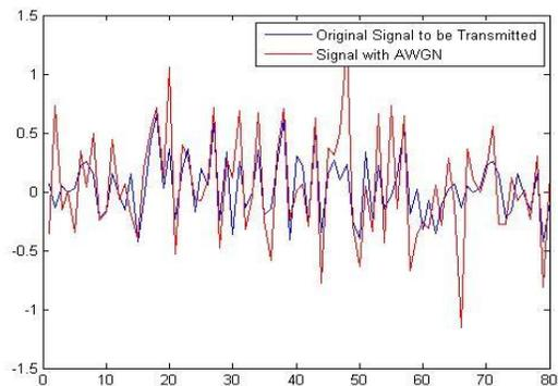
Fig: 4(e). Noise Added Transmitted Signal
