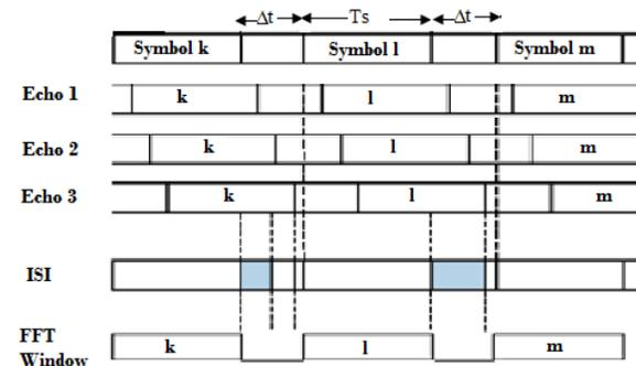
Fig. 3 (a). Combining ISI using a Guard Period [1]
