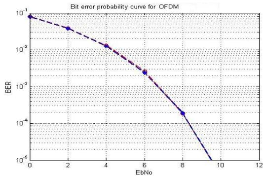
Fig: 4(c). BER of AWGN Channel
