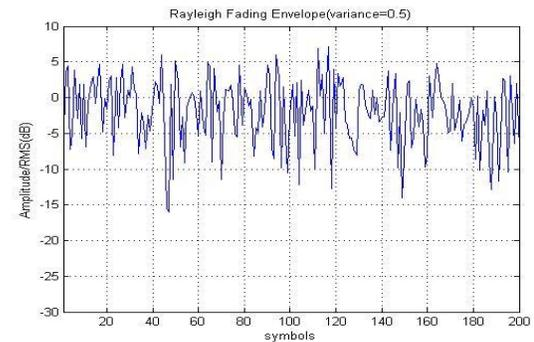
Fig: 4(i). Rayleigh Multipath Channel with AWGN Fading Envelope
