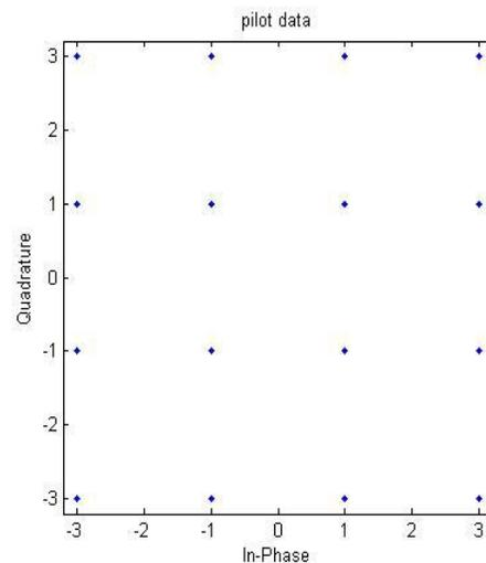
Fig: 4(a). Transmitted 16-QAM Constellation Diagram
