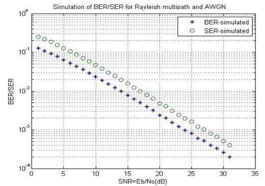
Fig: 4(h). BER and SER of Rayleigh Multipath Channel with AWGN Channel
