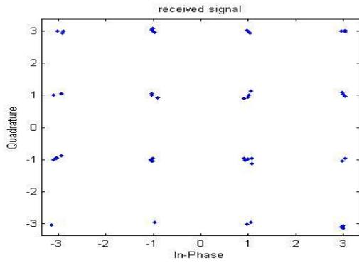
Fig: 4(b). Received 16-QAM Constellation Diagram
