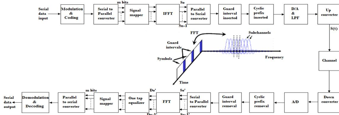
Fig. 1. Block Diagram of OFDM System
