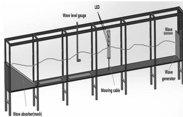
**Fig. 1.** Schematic View of the Wave Generation Wave Flume
