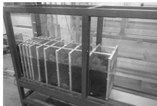
**Fig. 2.** The Snapshots Of The Wave Absorber
