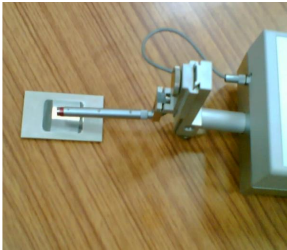
Fig: 10. Calibrating view with Measuring Instrument (Surtronic 3+)
