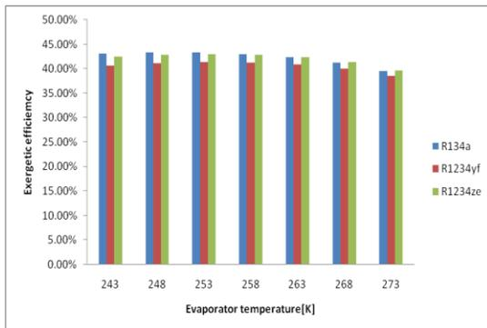
Fig. 3. Variation of exergetic efficiency with evaporators' temperatures
