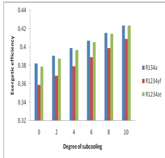
Fig. 6. Variation of exergetic efficiency with degree of sub cooling at condenser outlet
