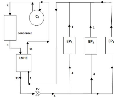
**Fig: 1(a).** Schematic diagram of actual multi evaporator with single compressor and single expansion valve and LVHE
