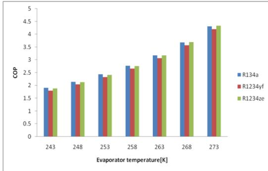
Fig. 2. Variation of COP with evaporators' temperatures
