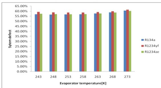
Fig. 4. Variation of system defect with evaporator temperatures
