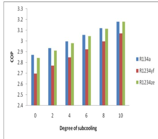
Fig. 5. Variation of COP with degree of sub cooling at condenser outlet
