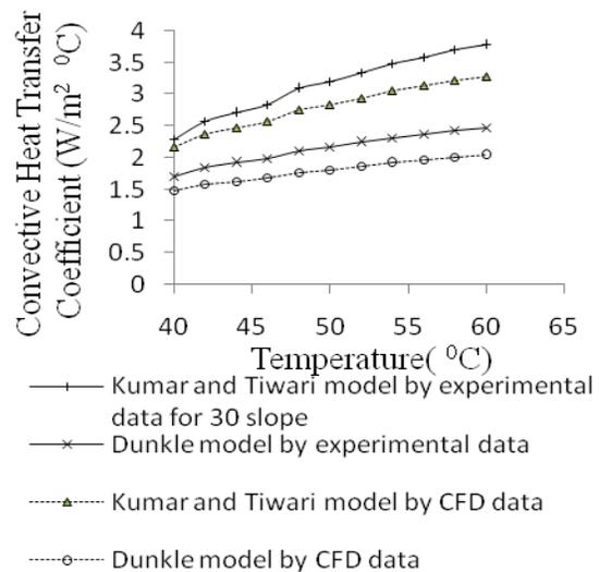
**Fig. 14.** Variation of (h<sub>cv</sub>) within temperature range of 400- 600C for 300 slope of the condensing cover
