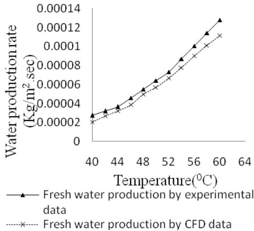
Fig. 7. The rate of fresh water production from experimental data and simulation result for 150 inclination
