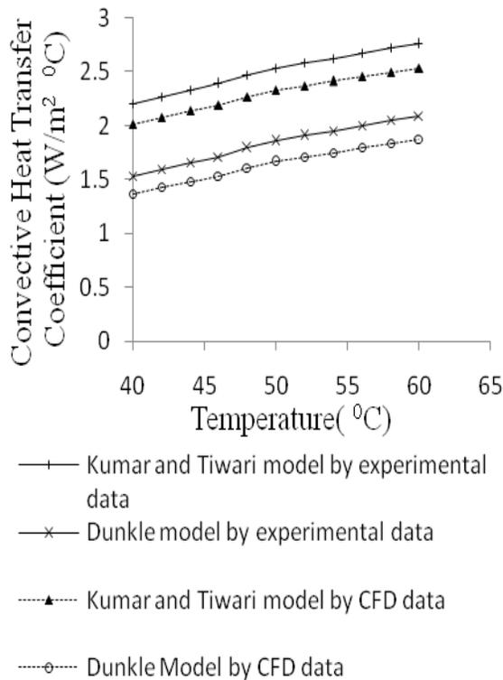
**Fig. 12.** Variation of (h<sub>cv</sub>) for 150 slope of the condensing cover
