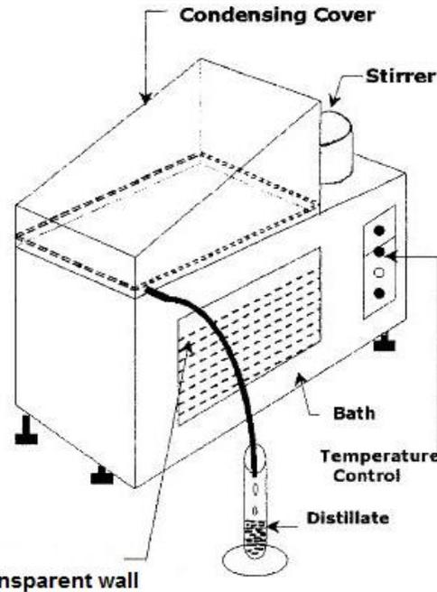
**Fig: 1.** A schematic diagram of experimental setup of solar still [4]
