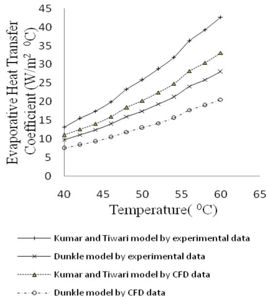
**Fig: 15.** Variation of evaporative heat transfer coefficient (hew) within temperature range of 400- 600C for 300 slope of the condensing cover
