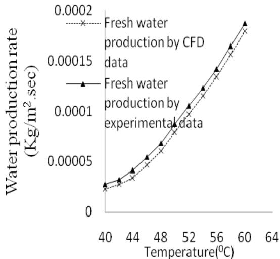
Fig. 8. The rate of fresh water production from experimental data and simulation result for 300ininclination
