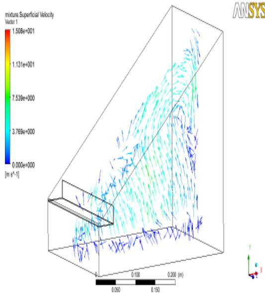
**Fig. 11.** Gas mixture velocity on a plane inside the solar still for 300in inclination
