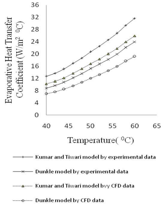
**Fig. 13.** Variation of evaporative heat transfer coefficient (h<sub>ew</sub>) within temperature range of 400- 600C for 150 slope of the condensing cover
