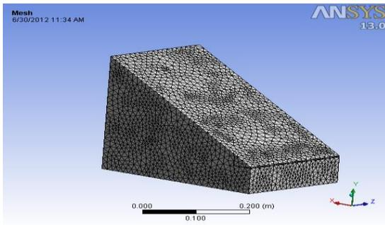
Fig. 2. 3D Unstructured mesh for 150ininclination
