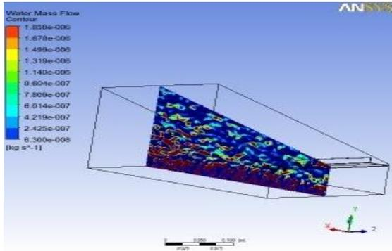
Fig. 6. Water mass flow predicted by CFD simulation.
