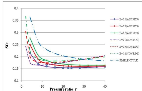
**Fig. 10.** Effect of Pressure Ratio on Specific Fuel Consumption with Effectiveness [ $T_1=300$  K,  $TIT=1500$  C]
