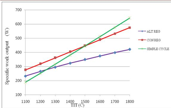
**Fig. 12.** Effect of TIT on Specific Work Output [ $T_1=300$  K,  $r = r_{opt}$ ]
