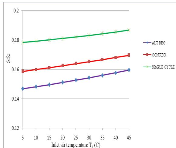
**Fig. 16.** Effect of the Inlet Air Temperature on Specific Fuel Consumption [ $TIT = 1500$   $^{\circ}$ C,  $r = r_{opt}$ ]
