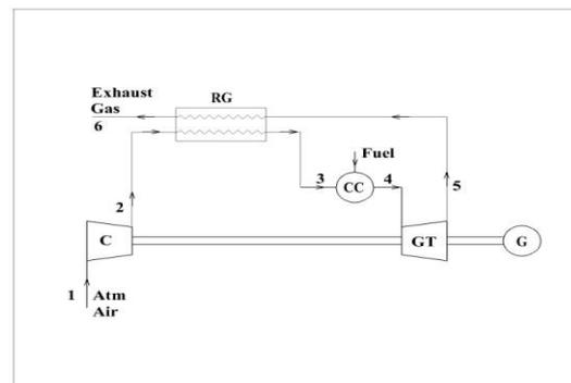
Fig. 2. Schematic diagram of gas turbine regenerative cycle
