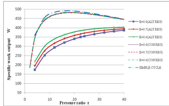
**Fig. 8.** Effect of Pressure Ratio on Specific Work Output with Effectiveness [ $T_1=300$  K,  $TIT=1500$  C]
