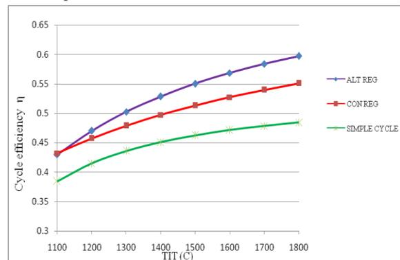
**Fig. 11.** Effect of TIT on efficiency [ $T_1=300$  K,  $r = r_{opt}$ ]
