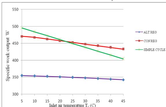
**Fig. 15.** Effect of the Inlet Air Temperature on Specific Work Output [ $TIT = 1500$   $^{\circ}$ C,  $r = r_{opt}$ ]
