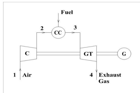
Fig. 1. Schematic Diagram of Simple Gas Turbine Cycle
