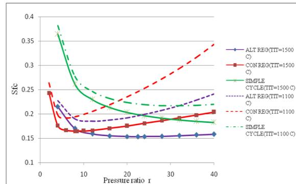
**Fig. 9.** Effect of Pressure Ratio on Specific Fuel Consumption with TIT [ $T_1=300$  K,  $E=0.8$ ]
