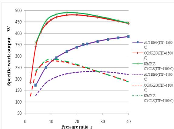
**Fig. 7.** Effect of Pressure Ratio on Specific Work Output with TITs [ $T_1=300$  K,  $E=0.8$ ]
