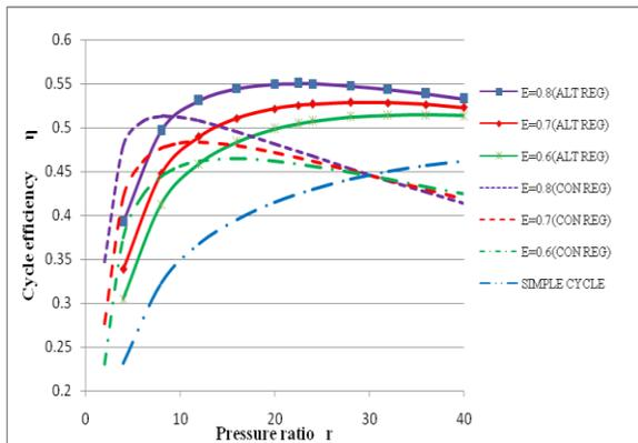
**Fig. 6.** Effect of Pressure Ratio on Efficiency with Effectiveness [ $T_1=300$  K,  $TIT=1500$  C]
