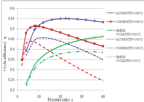
**Fig. 5.** Effect of Pressure Ratio on Cycle Efficiency with TIT [ $T_1=300$  K,  $E=0.8$ ]
