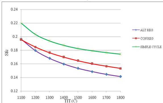
**Fig. 13.** Effect of TIT on Specific Fuel Consumption [ $T_1=300$  K,  $r = r_{opt}$ ]
