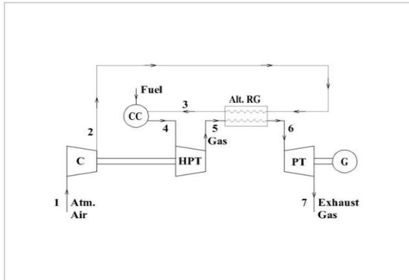
**Fig. 3.** Schematic Diagram of Gas Turbine with Alternative Regeneration Cycle
