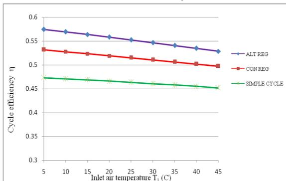
**Fig. 14.** Effect of the Inlet Air Temperature on Efficiency [ $TIT = 1500$   $^{\circ}$ C,  $r = r_{opt}$ ]
