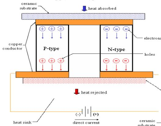
Fig. 2. Current Flow in P-N Junction
