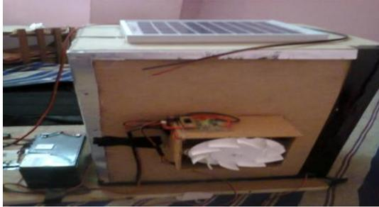
**Fig. 4.** Working Model of a Compressor less Solar AC
