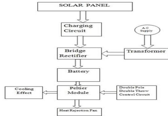
Fig. 3. Block diagram of the solar AC
