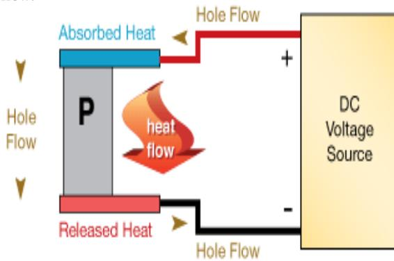
Fig. 1. Supply in P-Type Semiconductor
