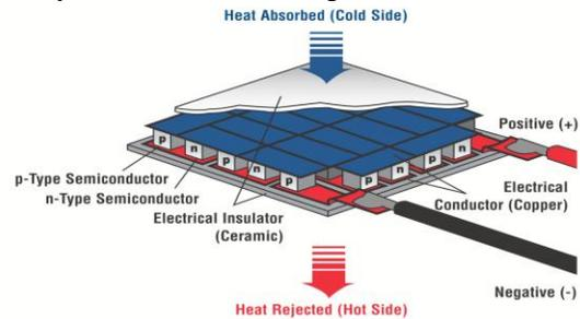
**Fig. 5.** A Cutaway of Thermoelectric Module
