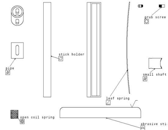
**Fig. 6.** Different parts of a honing tool
