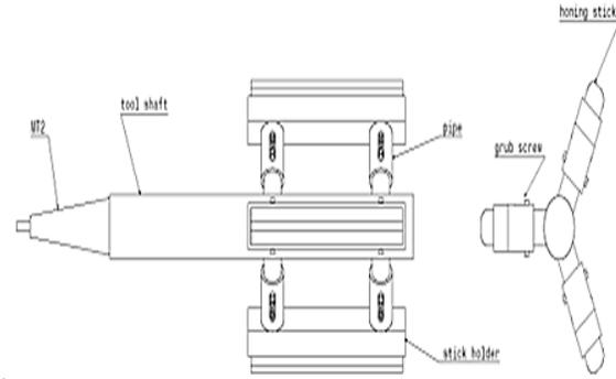
**Fig. 5.** Honing tool for a drilling machine
