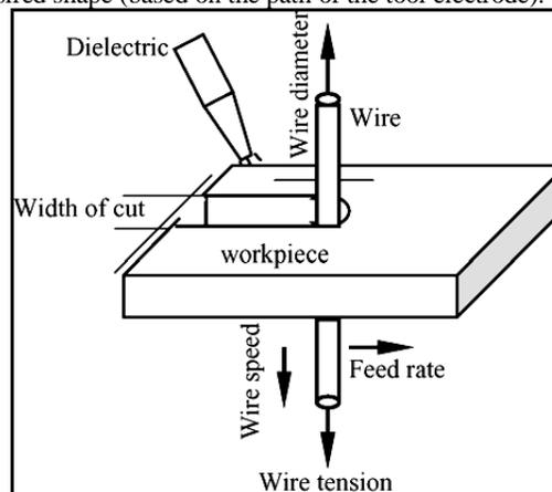
Fig. 1. Wire-EDM process [6]
