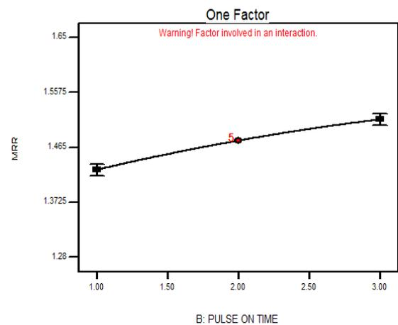
**Fig. 8.** Effect of Pulse on time on MRR
