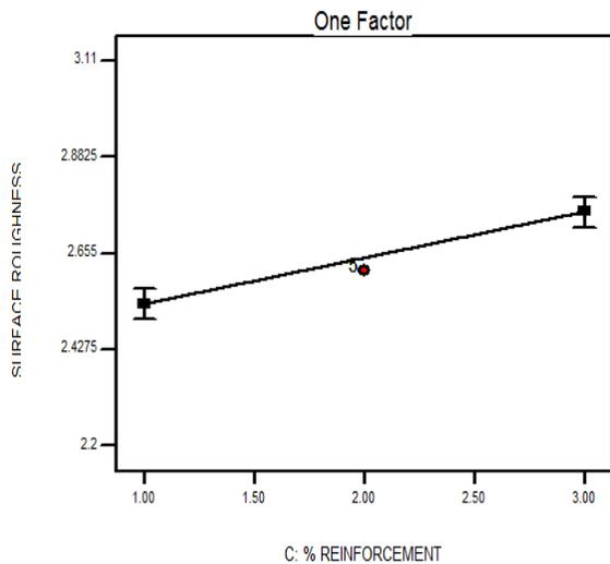
**Fig. 6.** Effect of Reinforcement on Surface Roughness
