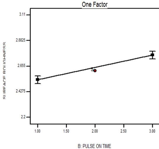
**Fig. 5.** Effect of Pulse on time on Surface Roughness
