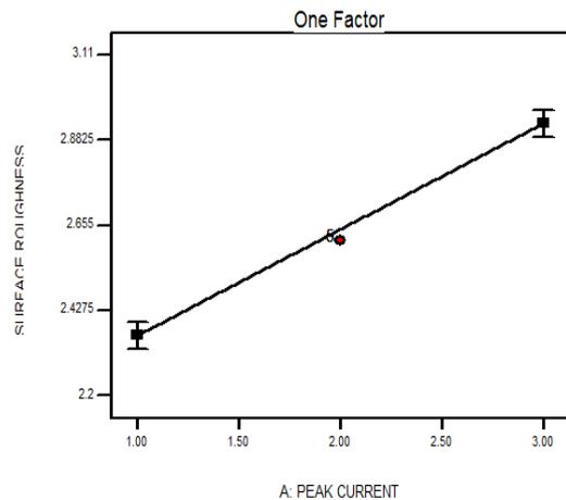
Fig. 4. Effect of peak current on Surface Roughness
