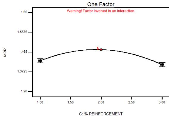
**Fig. 9.** Effect of % Reinforcement on MRR
