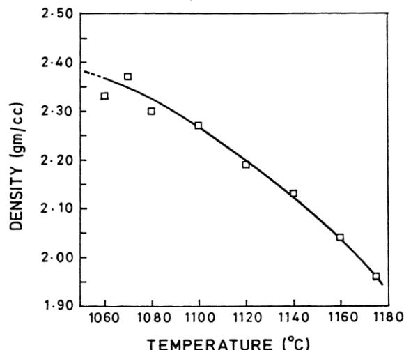
**Fig. 1.** variation of density with sintering temperature for MAS glass ceramic prepared by sintering route [1]
