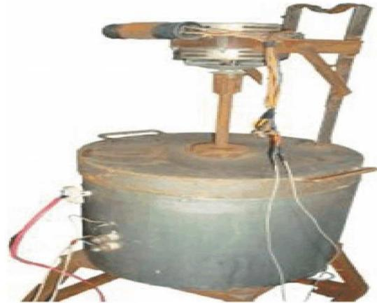
**Fig: 5.** Stir Casting Unit [7]
