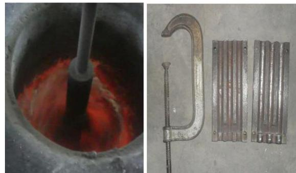
Fig. 4. Preparation of Al-5083 composite & CI permanent mould [5]
