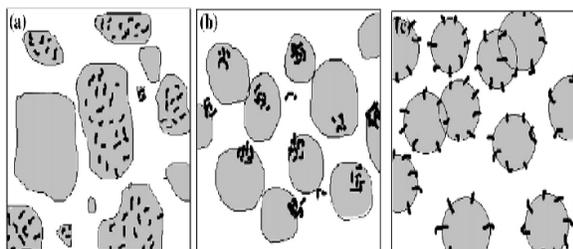
**Fig: 6.** Schematic depictions of CNTs and Al powder after different mixing techniques. In (a) high energy ball milling, CNTs were effectively dispersed though insufficiently distributed within the Al powders; and in (b) low energy ball milling, CNTs dispersed within Al powder though agglomerates still existed; and in (c) the PBA method, CNTs were coated with Al powders though agglomerates still existed. [10]
