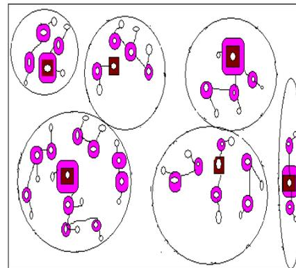
At this level, Sub cluster Head transmit their data to the nearest Sub Cluster Head in parallel way. this process will continue until all the data has to be transmitted to the Sub Cluster Head.
