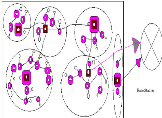
Data aggregation function will be implemented at this level by each Cluster head and then transmit the data to nearest Cluster Head if the distance between Cluster head and base station is less as comparison to another cluster head then this cluster head transmit their data to the base station directly.
