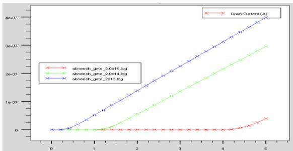
**Fig: 2.** Characteristics curve of  $V_{gs}$  Vs  $I_d$  having concentrations  $2 \times 10^{15}$ ,  $2 \times 10^{14}$  and  $2 \times 10^{13}$
