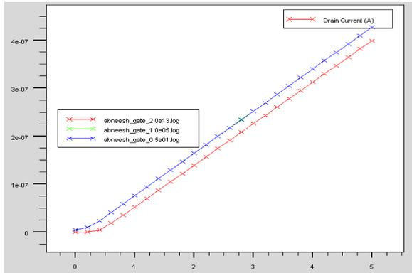
**Fig: 4.** Characteristics curve of  $V_{gs}$  Vs  $I_d$  having concentrations  $2 \times 10^{13}$ ,  $1 \times 10^5$  and  $0.5 \times 10^1$
