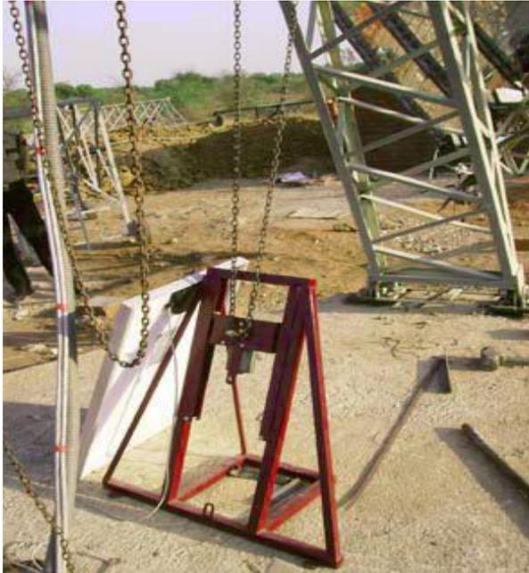
**Fig. 3.** Automatic tracking Stand for small Scheffler reflector
