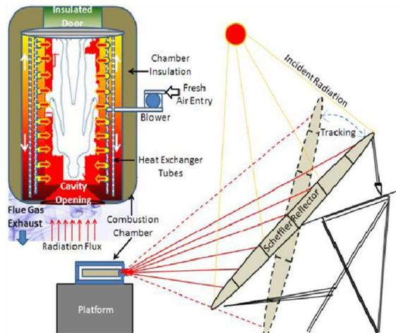
Fig. 1. Block Diagram of Solar Crematorium
