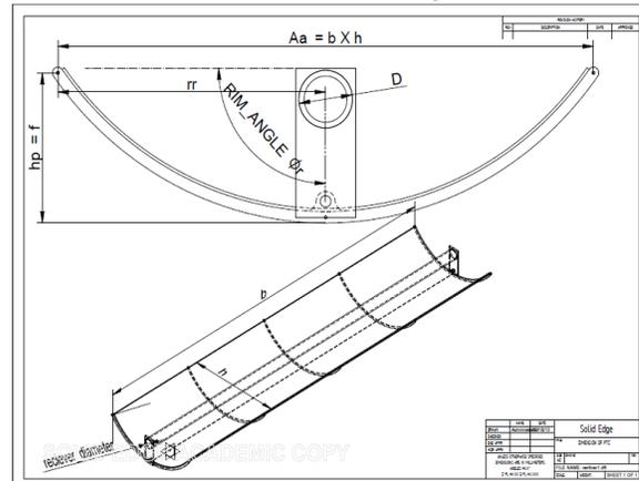
**Fig. 3.** Schematic of parabolic through collector.
