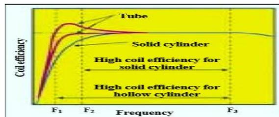
Fig. 5. Graph coil efficiency vs. frequency conditions for maximizing the electrical efficiency of the induction coil are different for tubes and solid cylinders. [9]
