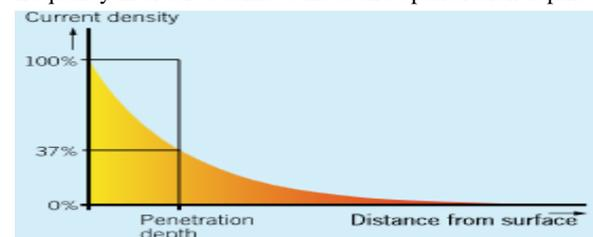
**Fig. 3.** graph current density vs distance from surface [9]
