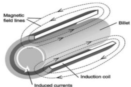
**Fig. 2.** Principles of induction heating of a massive cylinder (a billet)
