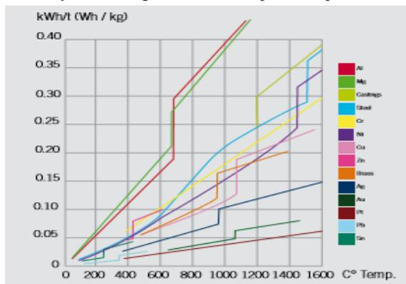
Fig. 4. Energy requirement rate for different materials [9]
