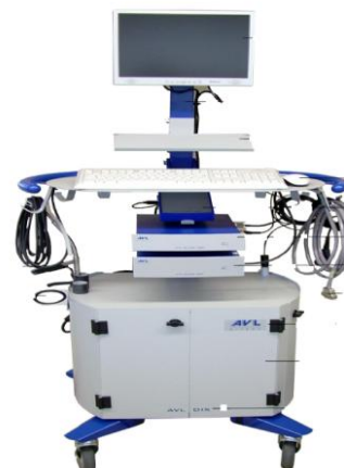
Fig. 3. Emission Test Machine used in Bio Diesel Emission
