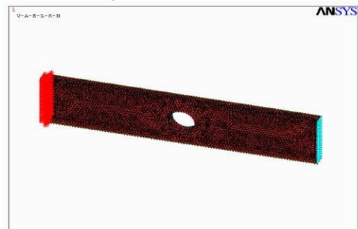
**Fig. 2.** Application of Boundary Condition
