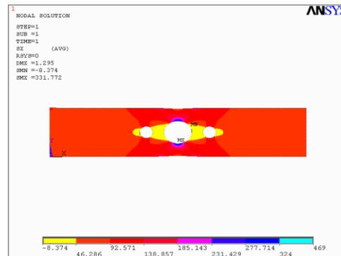
Fig. 11. Stress Plot at Mesh Size 2
