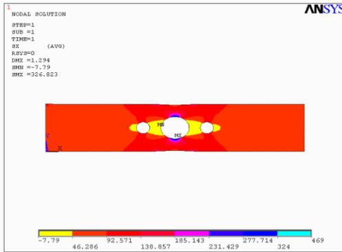
Fig. 5. Stress Plot at Mesh Size 6
