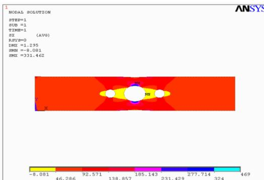
Fig. 7. Stress Plot at Mesh Size 3
