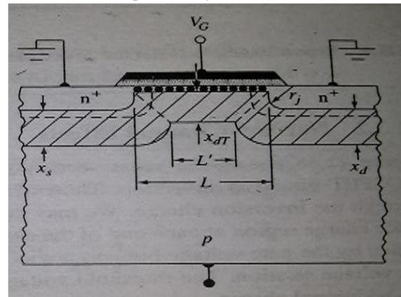
Fig. 2. Charge Sharing in the Short Channel Threshold Voltage Model
