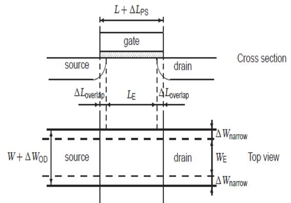
Fig. 1. Cross Section View of MOSFET
