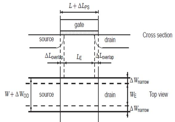
Fig. 1. Cross Section View of MOSFET
