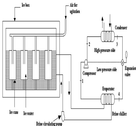
**Fig: 1a.** Schematic Diagram of an Industrial Ice Plant
