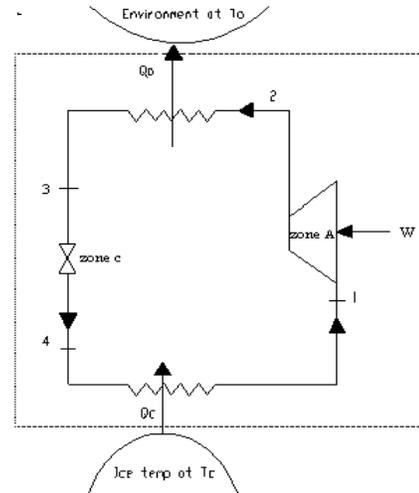
**Fig: 1a.** Schematic Diagram of an Industrial Ice Plant
