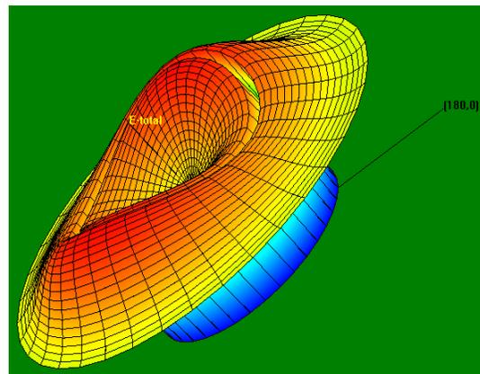
**Fig. 9.** 3d Radiation Pattern of back to back E shape Antenna
