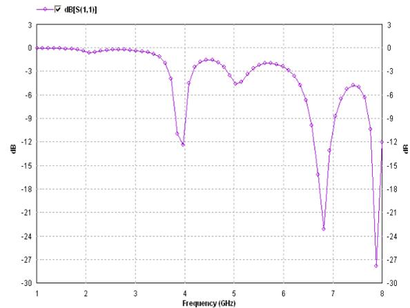
Fig: 3. Return loss Vs Frequency Curve of Microstrip Patch Antenna with back to back E Shape Slots Antenna
