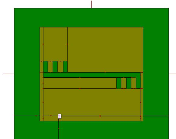
Fig: 2. Microstrip Patch Antenna with back to back E shape slots Feed at (-7.57, -13.35).
