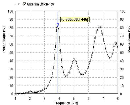
**Fig. 7** Antenna Efficiency Vs Frequency Curve
