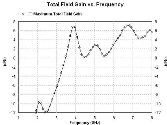
**Fig. 5.** Total Field Gain Vs Frequency Curve
