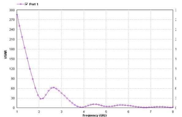
Fig: 4. VSWR Vs Frequency Curve
