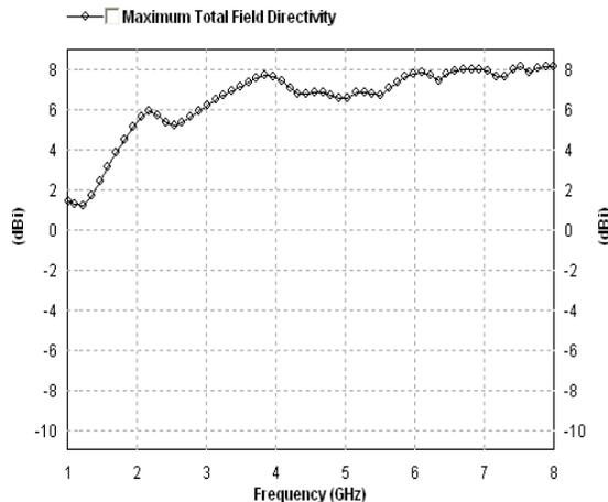
**Fig. 6** Directivity Vs Frequency Curve
