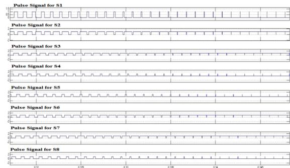
**Fig. 9.** Eight gating signals for firing the cascade H-bridge Inverter
