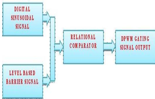
Fig. 3. Model for PWM Signals Generation
