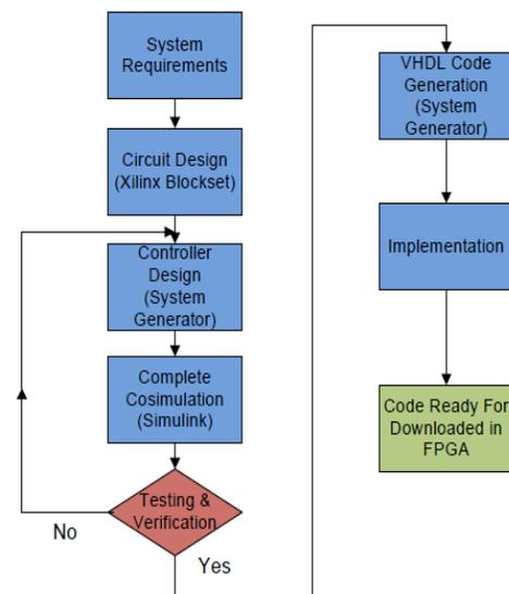
Fig. 5. Design flow diagram for MATLAB/Simulink and Xilinx System Generator
