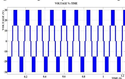
**Fig. 7.** Five-Level Cascade Multilevel Inverter Output Waveform
