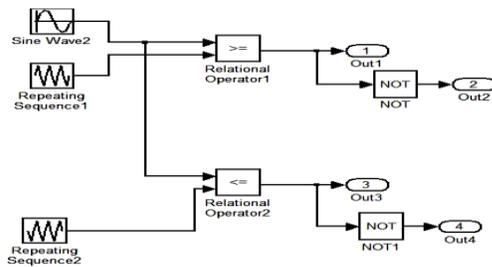
**Fig. 6.** Circuit Diagram of Pulse Generator
