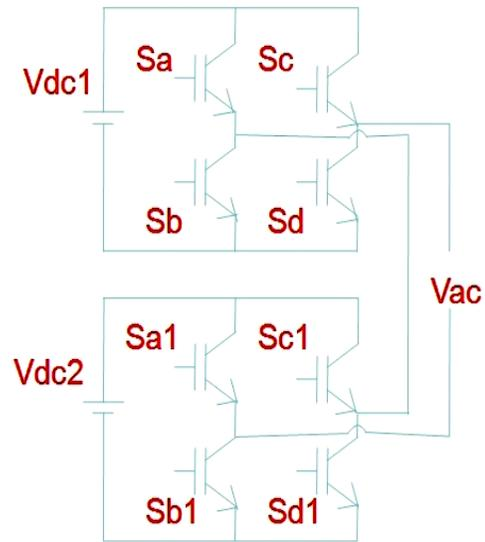
Fig. 2. The cascaded H-bridge multilevel inverter circuit
