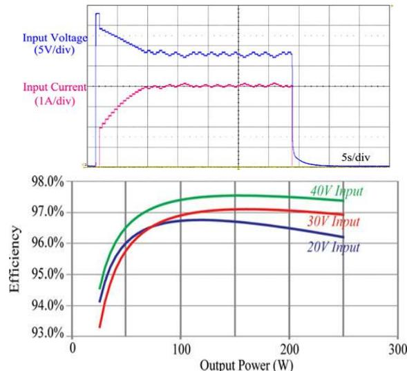
Input voltage and current during startup, P&O MPPT, and shutdown using a BP Solar SX6165N 165-W PV Panel (112-W operating power) (400-Vdc output). Projected power stage efficiency (400-Vdc output)
