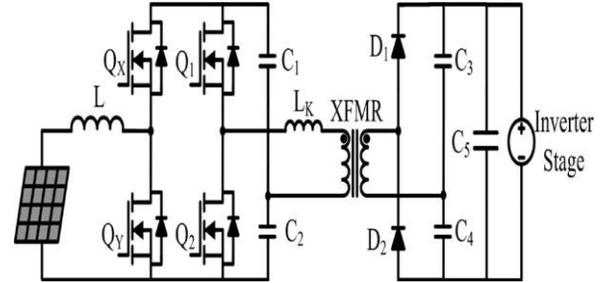
Fig. 2. Resonant half-bridge with separate boost input stage.
