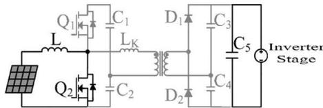
$$T_{res2} = \pi \sqrt{\frac{L_k C_2 n^2 (C_3 + C_4)}{C_2 + n^2 (C_3 + C_4)}}$$
