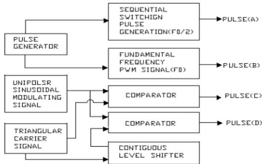
Fig: 6. Base modulation generator – HSCPWM
