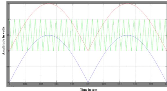
**Fig: 3.** Waveform pattern for SCSPWM scheme
