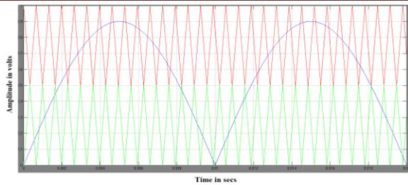
**Fig: 2.** Waveform pattern for APOD scheme
