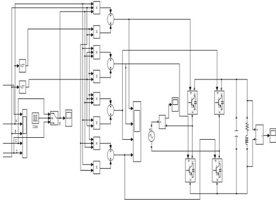
**Fig: 10. Logical Simulation Diagram - Gate Pulses**
