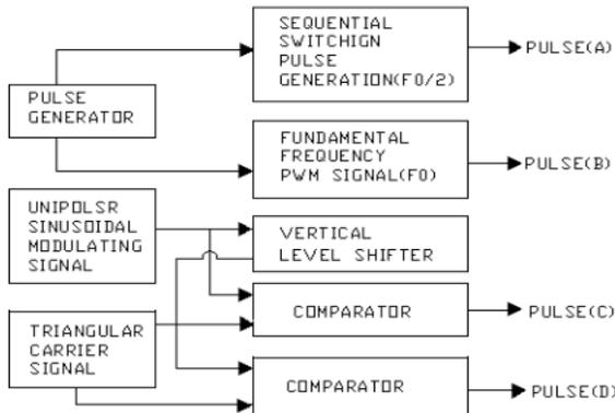
Fig: 7. Base modulation generator – HSCPWM
