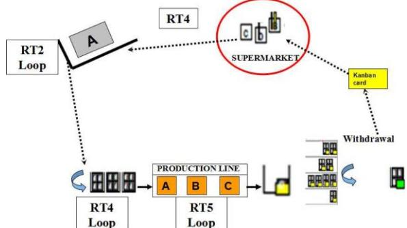
**Fig: 4** Schematic Representation of Lot Size Coverage Factor in Kanban Calculation
