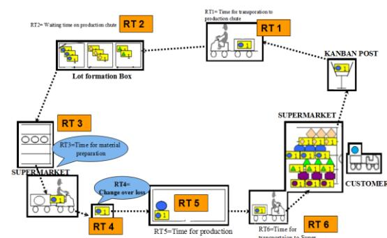
**Fig: 1** Schematic Representation of RT loop in kanban Calculation
