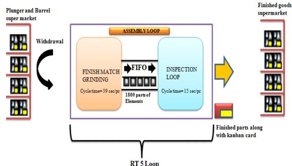
**Fig: 3** Production Time for 1 Kanban Quantity
