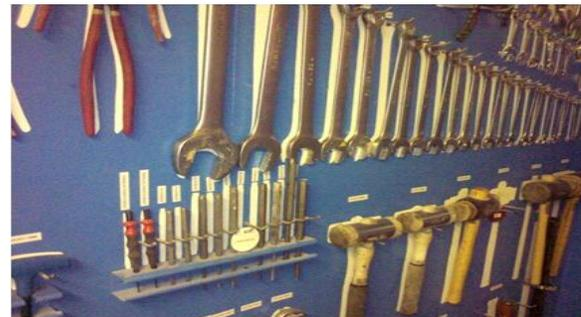
**Fig. 2.** Shadow Board Displaying all the Equipment and tools at its Right Place
