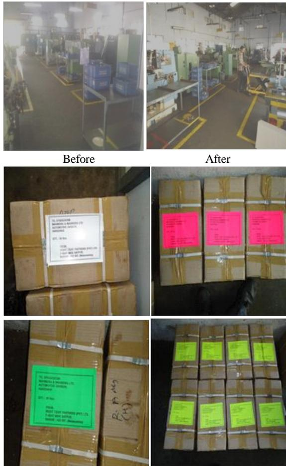
**Fig: 10.** Marking and Standardization of the Templates with different color codes. (each color code specifies a particular company/product which helps in minimizing the problem of dispatching the different product to other company).
