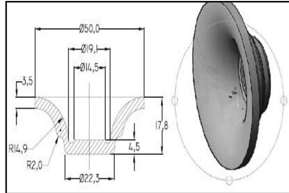
Fig. 1. Selected Component with Dimensions
