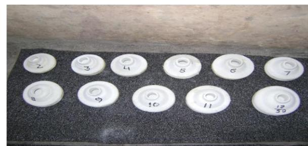
Fig. 4. Ready Shells for Pouring
