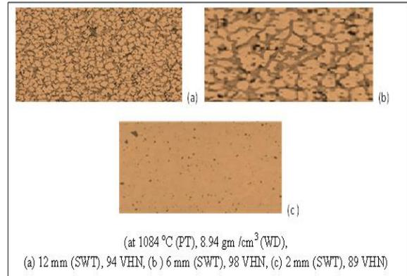
**Fig: 13.** Surface photomicrograph of Cu alloy casting
