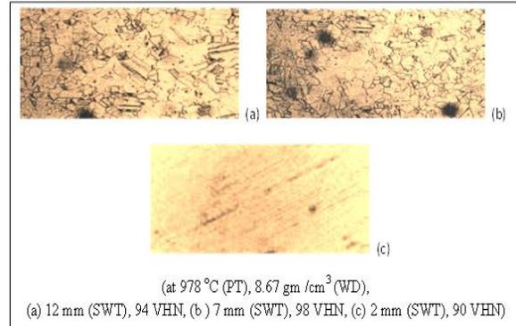
**Fig: 14.** Surface photomicrograph of brass alloy casting
