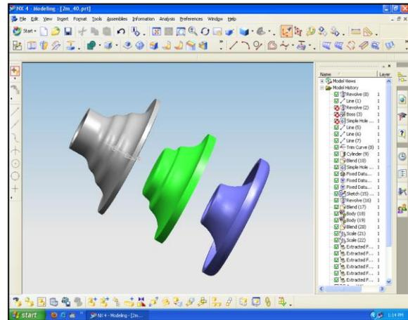
Fig. 2. CAD Model of Upper Shell, Component and Lower Shell
