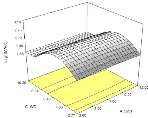
Fig. 8. Effects of SWT and WD on Vickers Hardness Number
