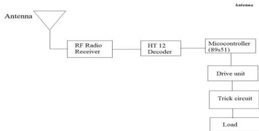
Fig. 1. Receiver module
