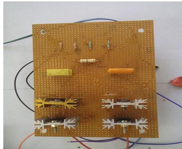
**Fig: 3.** Drive Control for Induction Motor
