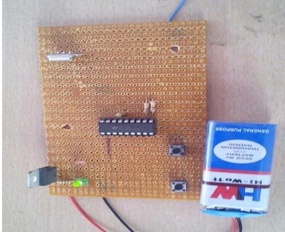
**Fig. 4.** Transmitter Section
