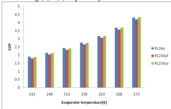
Fig. 1. Variation of COP with evaporators' Temperatures
