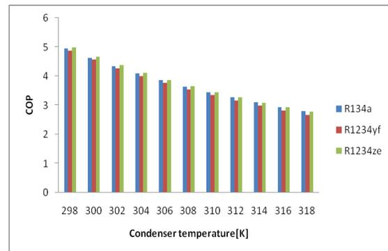
Fig. 6. Variation of COP with condenser temperature
