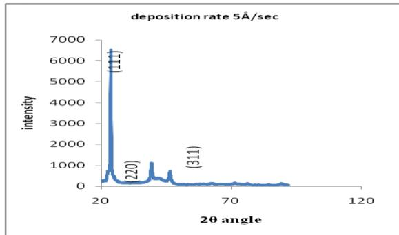
Fig: 3(b) CdTe deposition on Si at deposition rate of 5Å/sec
