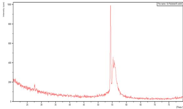
**Fig: 3(d).** XRD Analysis of Polished Silicon
