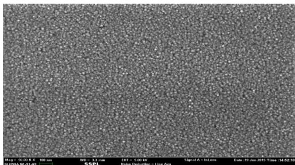
**Fig: 7(a).** SEM micrographs of CdTe at 50KX magnification with 5KV at deposition rate of 10 Å/sec
