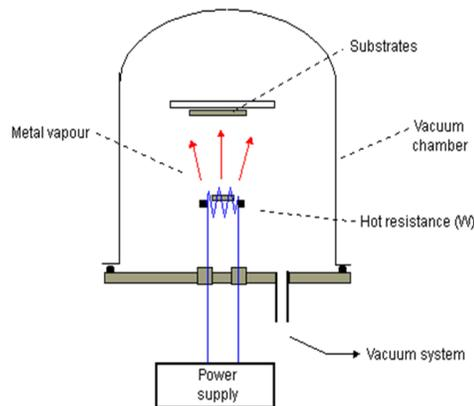
Fig. 1. Mechanism of Thermal evaporation process (ref. [8])
