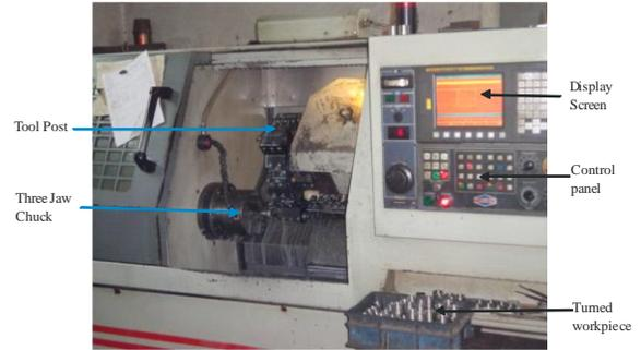
Fig 1 Photographic view of CNC Lathe machine
