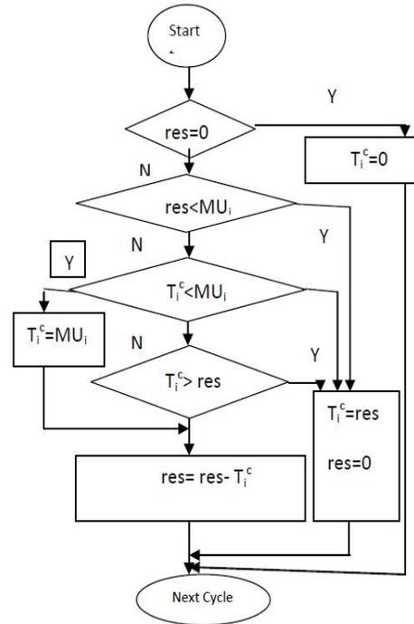
Fig. 2. Flow chart of modifying the cycles of unit
