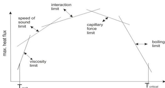
Fig. 3. Limitations of a Heat Pipe [2]
