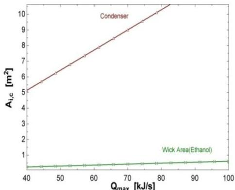
**Fig: 14.** Variation of Condenser area and wick area with heat capacity [8]
