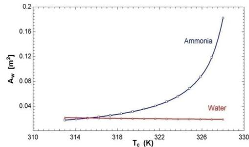
Fig. 6. Variation of Wick Area with operating temperature of heat pipe for Ammonia and Water [8]
