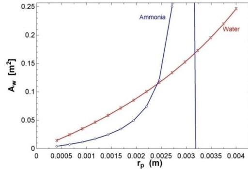
Fig 12: Plot between Wick Area and Pore Radius for Ammonia and Water [8]
