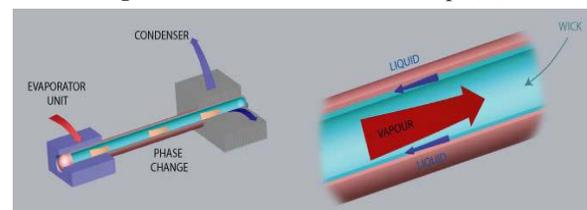
Fig. 2. Concept of Heat Pipe [2]
