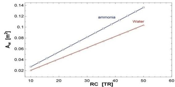
Fig. 7. Variation of Wick area with refrigerating capacity for Ammonia and Water [8]
