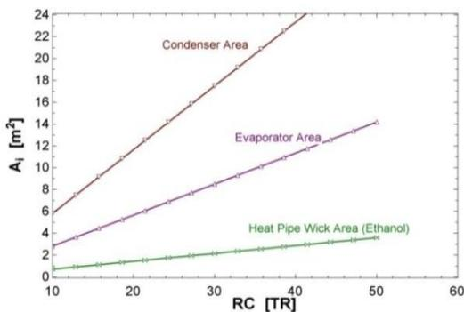
**Fig: 15:** Variation of condenser, evaporator and wick area with refrigerating capacity<sup>[8]</sup>
