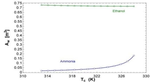
Fig. 5. Variation of Wick Area with operating temperature of heat pipe for Ethanol and Ammonia [8]
