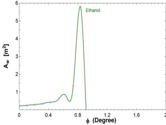
Fig 9: Variation of Wick Area with Inclination Angle for Ethanol [8]
