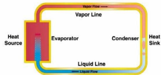
Fig. 1. Circular Process of a Heat Pipe [2]
