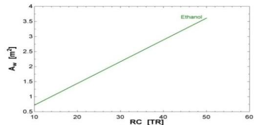
Fig. 8. Variation of Wick area with refrigerating capacity for Ethanol [8]
