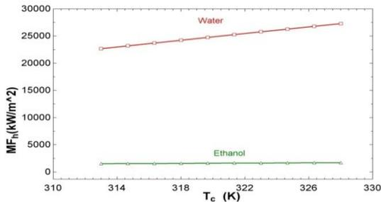
Fig. 4. Variation of Figure of Merit and Heat pipe temperature for Water and Ethanol [8]
