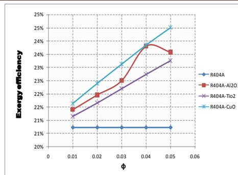
**Fig: 22.** Variation of Exergy Efficiency with volume fraction ( $\phi$ ) of VCERS with R404A using different nanoparticles
