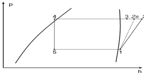
**Fig. 3.** Vapor Compression Cycle
