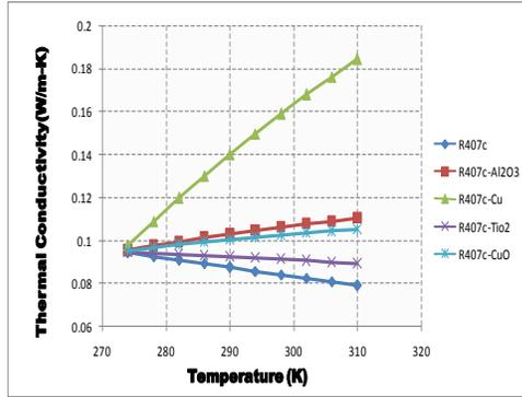
Fig: 5. Variation of Thermal conductivity with Temperature of R407c using different nanoparticles
