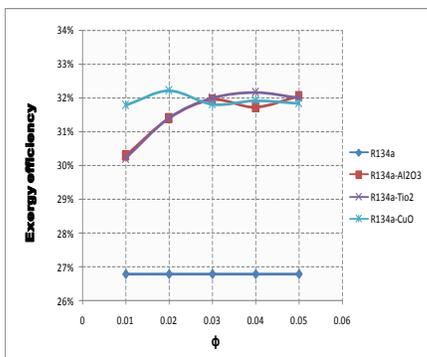
**Fig: 20.** Variation of Exergy Efficiency with volume fraction ( $\phi$ ) of VCERS with R134a using different nanoparticles
