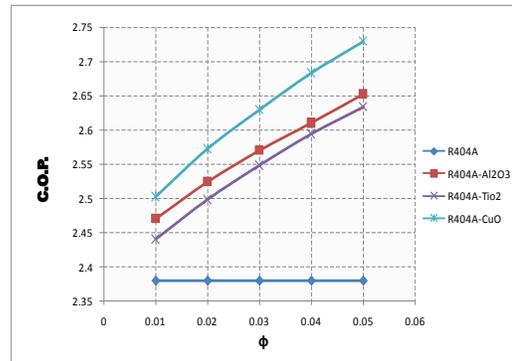
Fig. 16. Variation of C.O.P with volume fraction ( $\phi$ ) of VCRS with R404A using different nanoparticles
