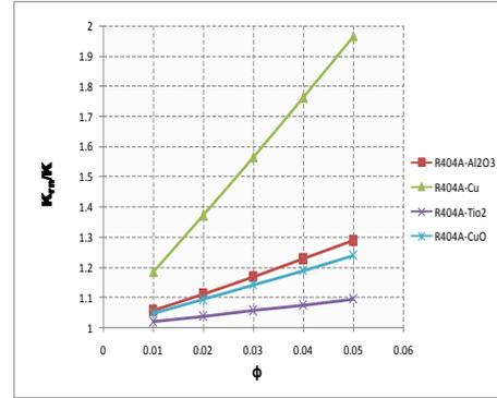
Fig: 8. Variation of Thermal conductivity Ratio with volume fraction ( $\phi$ ) of R404A using different nanoparticles
