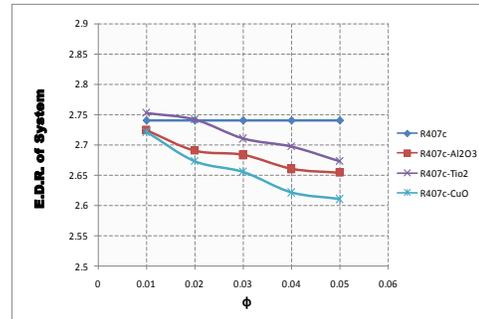
**Fig: 18.** Variation of Exergy Destruction ratio with volume fraction ( $\phi$ ) of VCERS with R407c using different nanoparticles
