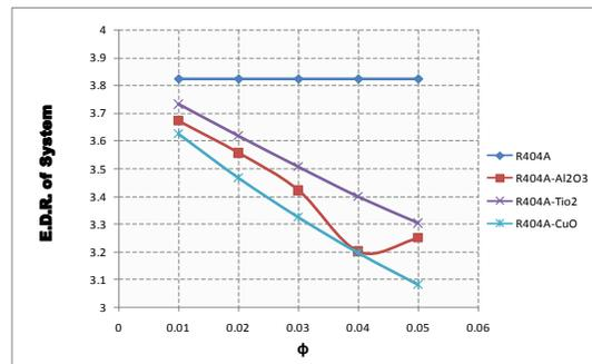
**Fig: 19.** Variation of Exergy destruction ratio with volume fraction ( $\phi$ ) of VCERS with R404a using different nanoparticles
