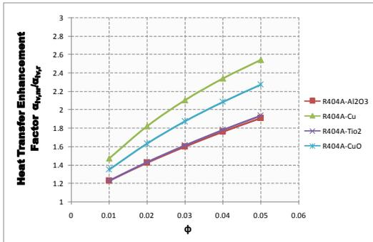
Fig. 12. Variation of Heat transfer Enhancement Factor with volume fraction ( $\phi$ ) of R404A using different nanoparticles
