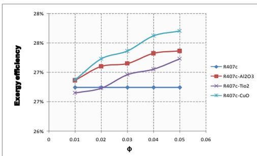
**Fig: 21.** Variation of Exergy Efficiency with volume fraction ( $\phi$ ) of VCERS with R407c using different nanoparticles
