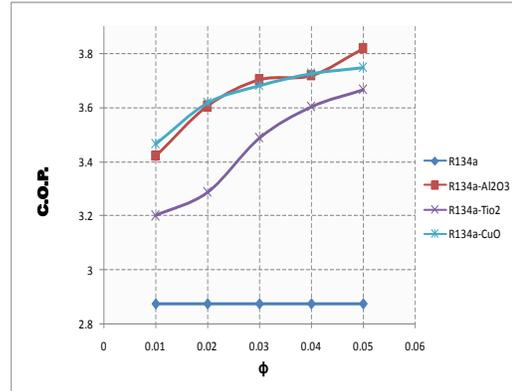
Fig. 14. Variation of C.O.P with volume fraction ( $\phi$ ) of VCRS with R134a using different nanoparticles
