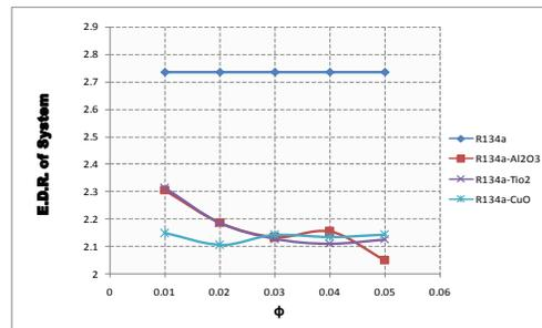
**Fig: 17.** Variation of Exergy destruction ratio with volume fraction ( $\phi$ ) of VCERS with R134a using different nanoparticles
