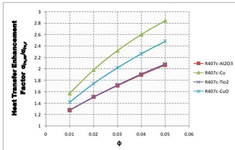
Fig. 13. Variation of Heat transfer Enhancement Factor with volume fraction ( $\phi$ ) of R407c using different nanoparticles
