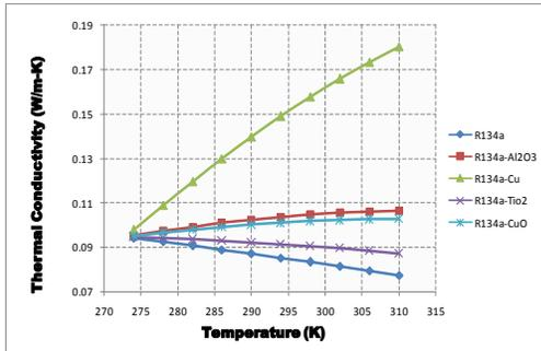
Fig: 6. Variation of Thermal conductivity with Temperature of R134a using different nanoparticles
