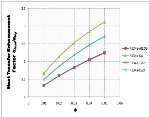
Fig. 11. Variation of Heat transfer Enhancement Factor with volume fraction ( $\phi$ ) of R134a using different nanoparticles
