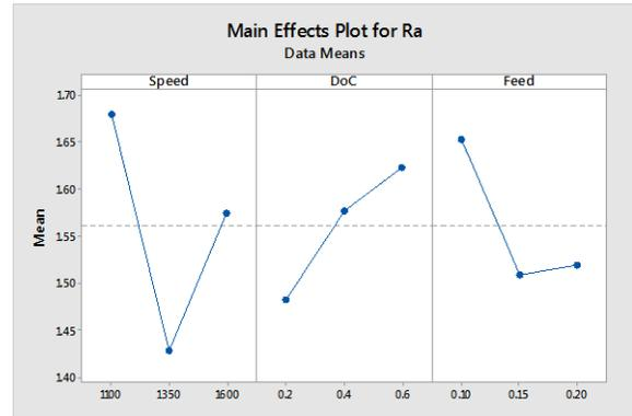
**Fig: 1.** Main effects plot for Ra
