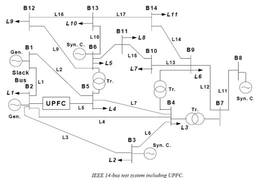
Fig. 2. One Line Diagram of 14 Bus System
