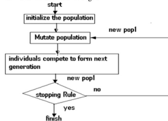
Fig. 1. Flow chart of Evolutionary programming
