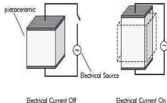
Fig. 1. An illustration of the Piezoelectric Effect
