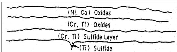
(c) Low temperature hot corrosion
