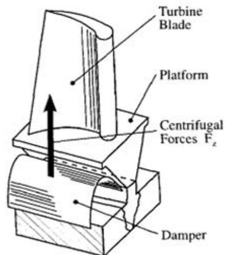
Fig. 1 Gas Turbine Blade
