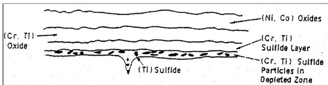
(b) Transition hot corrosion
