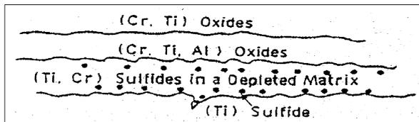
(a) High temperature hot corrosion
