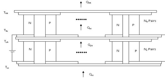
Fig. 1 Schematic diagram of the double stage TEC
