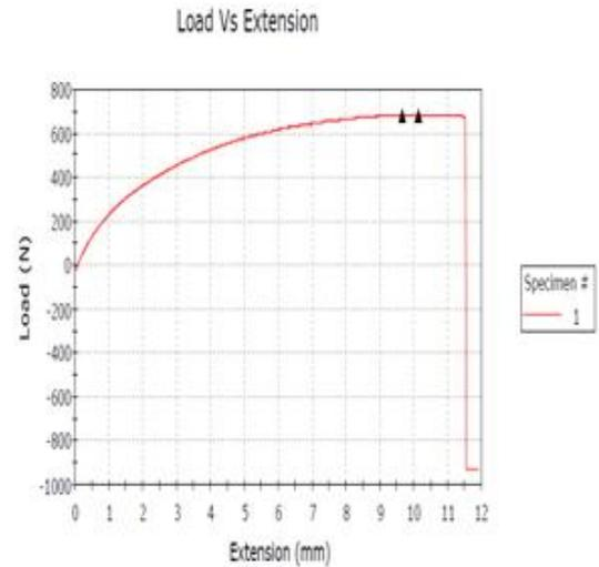
Fig. 4: Mechanical Properties at 14 W, Sample 1
