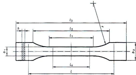
**Fig. 2: Shape and dimensions of the tensile test samples**
