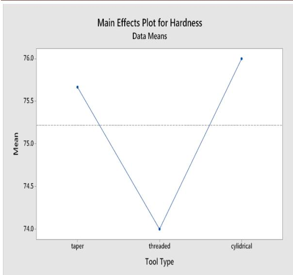
**Fig. 6.** Main Effects Plot for Hardness Vs Tool Type
