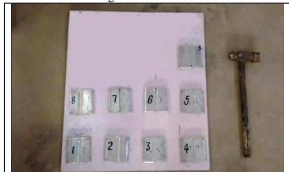
**Fig.3 Workpiece after FSW**
