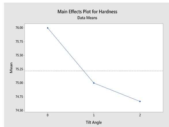
**Fig. 5.** Main effect plot for Hardness Vs Tilt Angle
