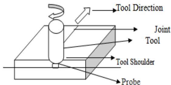
Fig.1 Friction Stir Welding Process
