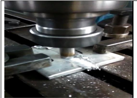
**Fig.2 FSW Set up**
