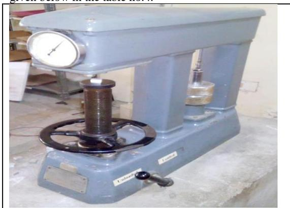
Fig. 4 Rockwell hardness machine
