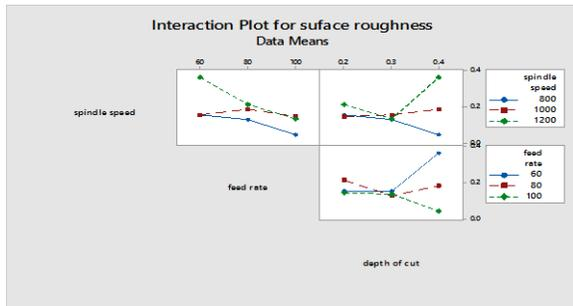
Fig. 5 Interaction Plot of All Factors for Surface Roughness
