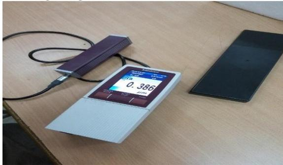
Fig.2 Mitutoyo Surftest SJ-201P Instrument
